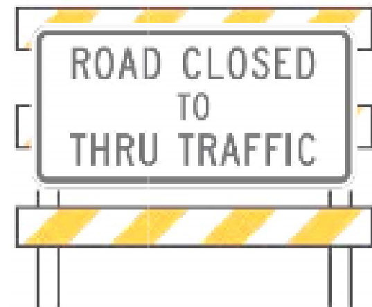
R11-4 on Type 3 Barricade with Two Steady Burn Warning Lights (60" Width)
